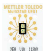
Flash DSC: MultiSTAR UFS 1 standard sensor or UFH 1 sensor for high temperature
