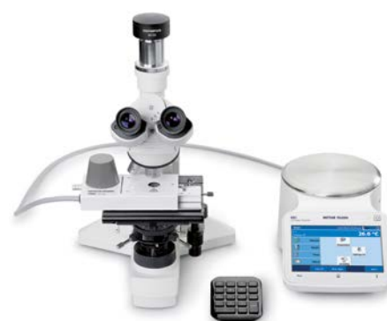
Microscope equipped with HS84 hot-stage
