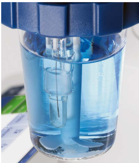
Compact G20S with manual titration kit and DGi115-SC sensor in a glass titration beaker
