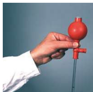
2. Intake by pressing on point B ↻
